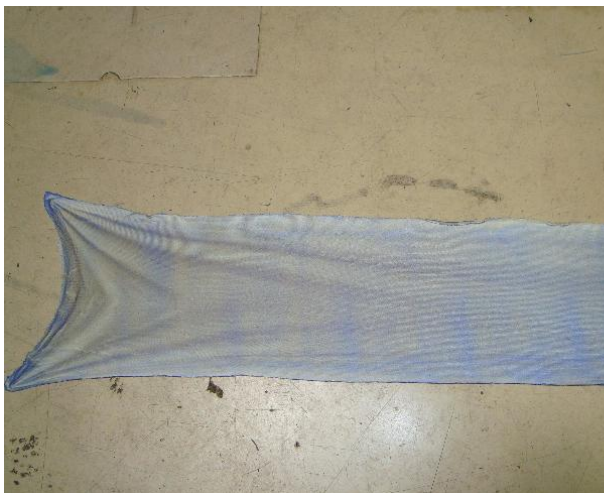
Figures 4: Bromophenol test (acetic acid in nitrogen): quasi homogeneous color (left) Bromothymol test ( \text{CO}_2 ): quasi homogeneous colour change to green (right)
