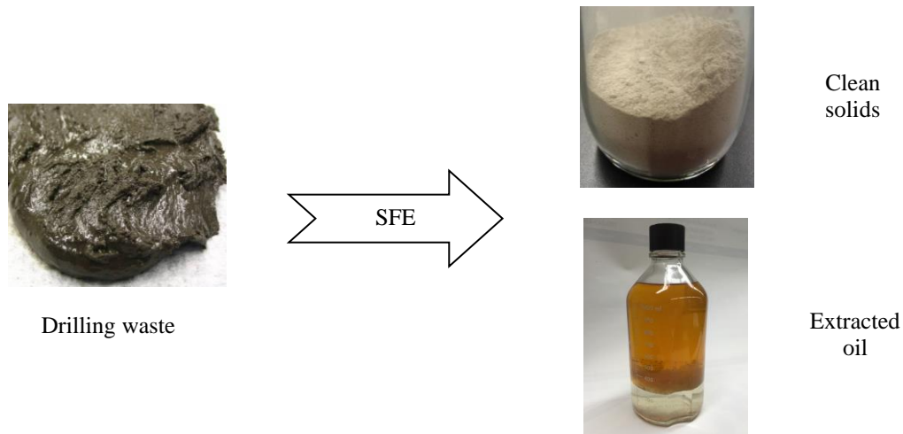
Figure 4. Extracted oil and clean solids after treating drilling waste with SC CO 2
