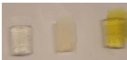
Figure 2 – Dry monoliths of silica gel impregnated by oil extracted from pulp by hexane: (a) as blank; (b) after direct impregnation; and, (c) after indirect impregnation.
