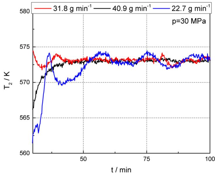
Figure 4: Temperature stability for  $T_2$  for different mass flow rates as a function of time [9]
