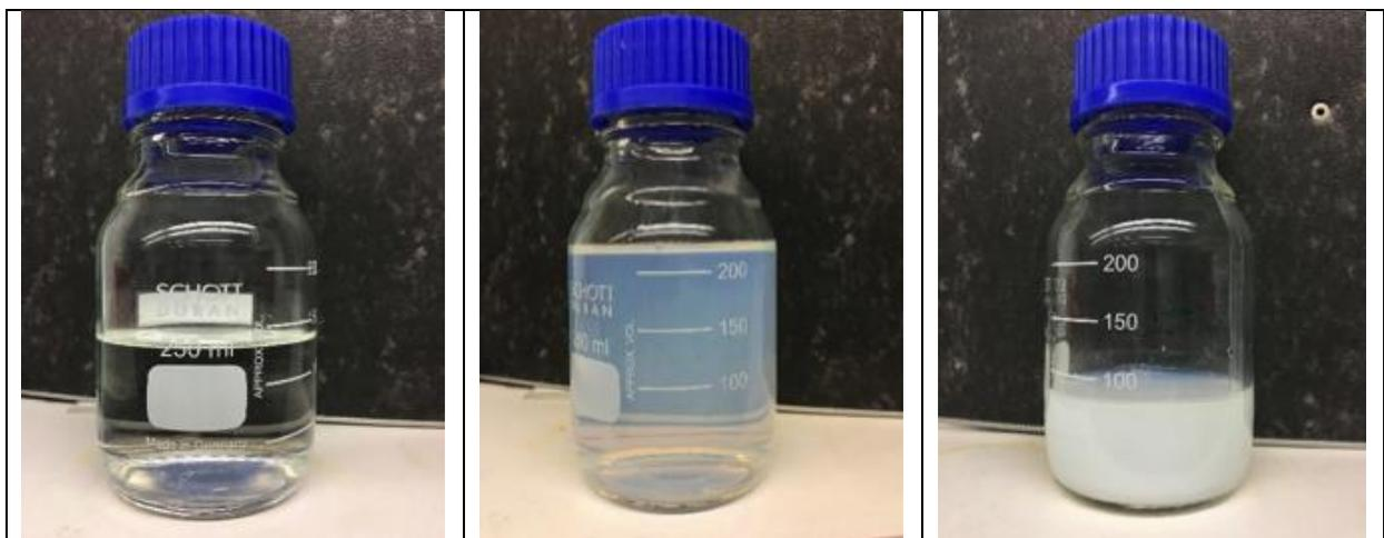
Figure 7: Suspensions obtained from different salt concentrations,  $0.005 \text{ mol l}^{-1}$ ,  $0.05 \text{ mol l}^{-1}$ ,  $0.15 \text{ mol l}^{-1}$  [9]
