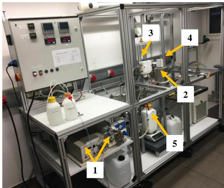
Figure 3: CHTS apparatus: 1 HPLC pumps, 2 heating unit, 3 isolated reactor, 4 cooler, 5 collection vessel
