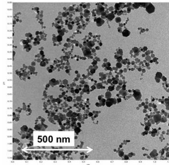
Figure 8:  $\text{CeO}_2$  nanoparticles (ca. 20-40 nm) synthesized at  $c_{\text{salt}} = 0.05 \text{ mol l}^{-1}$ ,  $\dot{m}_3 = 35 \text{ g min}^{-1}$ ,  $p = 30 \text{ MPa}$  and  $T_3 = 673 \text{ K}$  [9]
