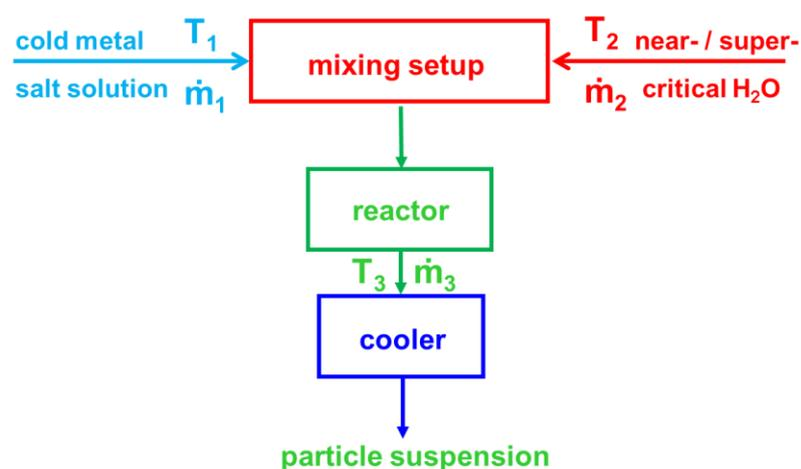
Figure 1: Basic principles of the CHTS process [3]
