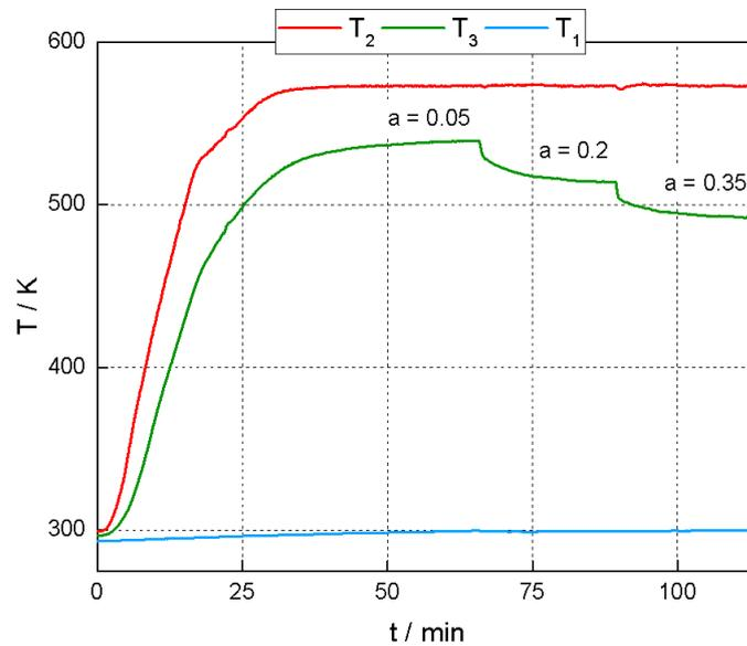
Figure 6: Process temperatures as a function of the time for different mixing ratios [9]
