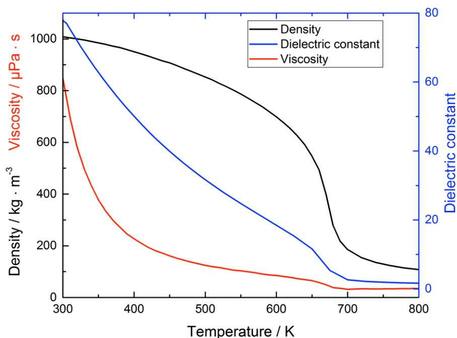
Figure 2: Changes in density  $\rho$ , viscosity  $\eta$  and dielectric constant  $\epsilon$  versus temperature at 25 MPa [3]
