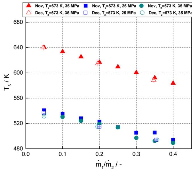
Figure 5: Mixing temperature  $T_3$  for different process conditions as a function of the mixing ratio  $a$  [9]
