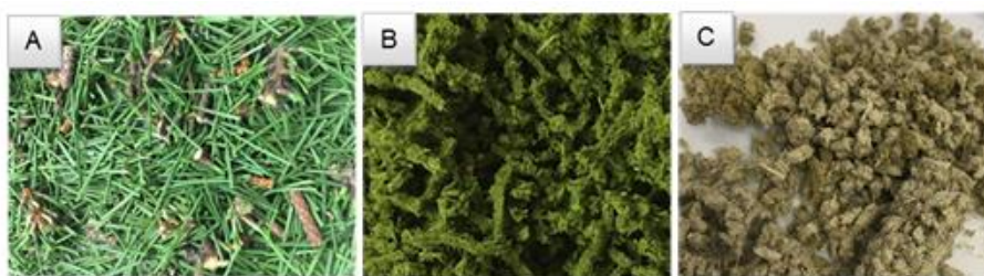
Figure 1. Pictures of the P. pinaster branches after being cut into portions of 2-4 cm (A); milled (< 2 mm) (B); and processed by scCO 2 extraction (C).
