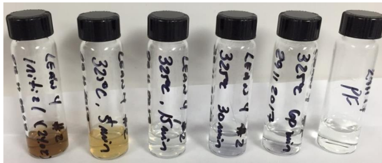
From left to right : CAW #4 sample before WAO and after 5, 15, 30, 60 min, and final purge
