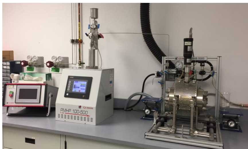
Figure 1: Wet air oxidation laboratory unit
