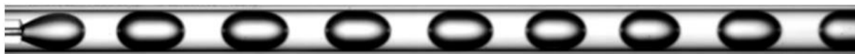
Figure IV. P = 20 MPa; T=308 K; V CO 2 = 0.02 mL.min -1 ; V H 2 O = 0.02 mL.min -1 in a 530 μm capillary.
